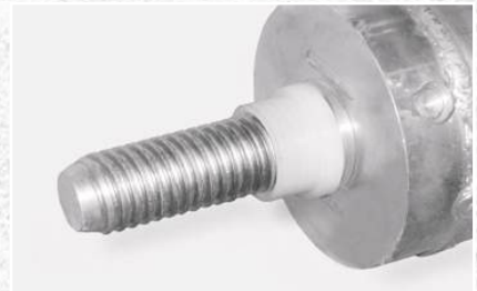
Install the UHMW bushing on the male end of the tube end.
