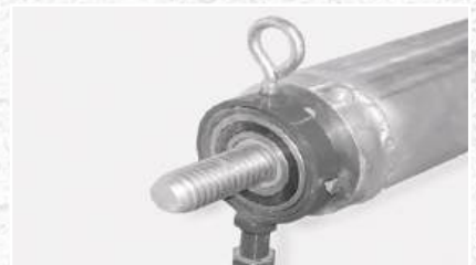
Remove pivot bearing from the centering tube and install on the UHMW bushing.
