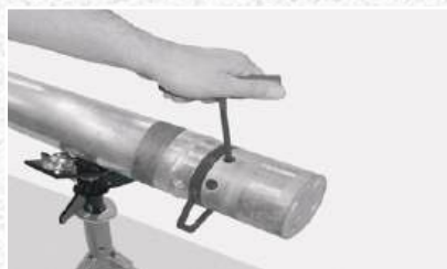
Use the tee handle tool provided to tighten the set screw.
