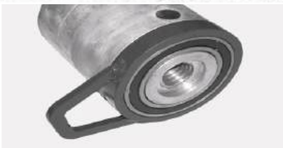
Install pulling eye bearing on wall plug.
